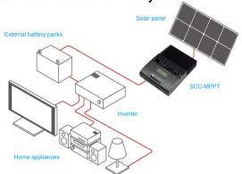
Combined MPPT technology and DSP controller, SCC-MPPT will convert best voltage to charge battery based on various temperature. Compared to traditional solar charge controllers, it allows your solar panels to operate at their optimum power output voltage, providing higher efficiency up to 98% with lower power loss.
