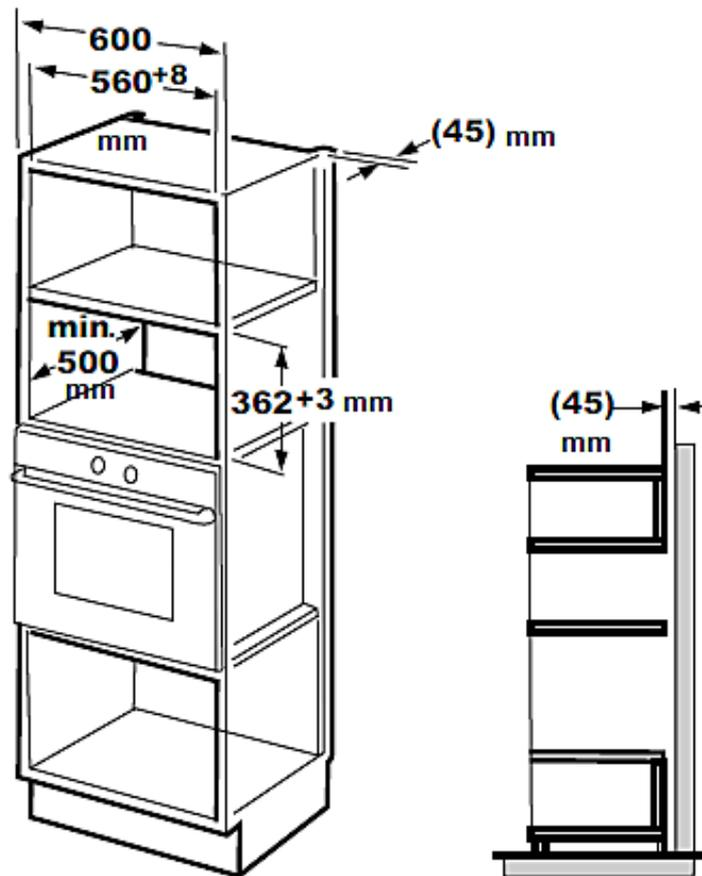
1. The piece of furniture the appliance is intended to be built-in **must not** be equipped with a back wall behind the appliance.
