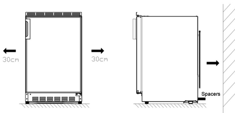
**i** Observe the required minimum distances for proper ventilation.
