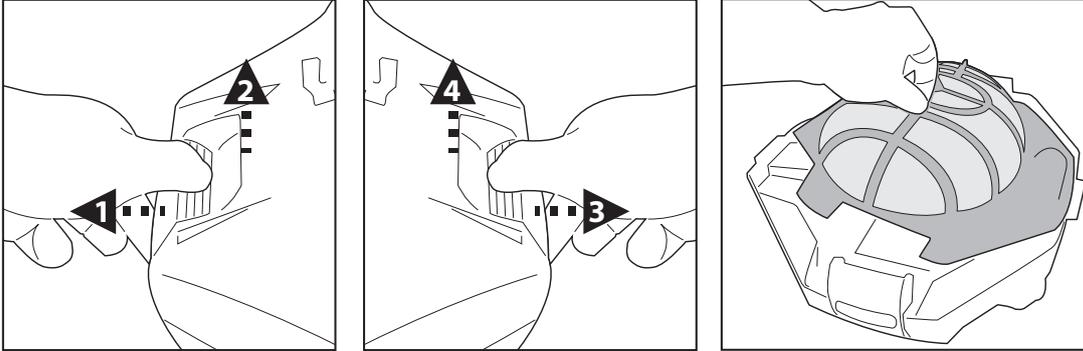
2. Detach the filter cover and remove the debris from the compartment. It is recommended to clean the filter cover net with splashing water. If brushing is deemed necessary, use only a soft brush to clean it carefully and gently to avoid damages.
