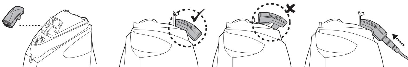
3. Connect the external adaptor to the power source. The indicator light on the external adaptor turns red once the charging begins. The indicator light on the external adaptor will turn green when the robot is charged.
