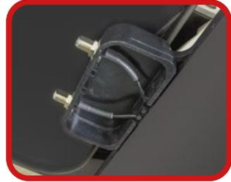
6. Then place the antenna on the mounting plate and fasten it again with the four Allen screws.
