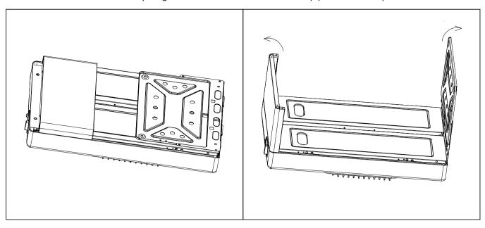
3.Open the side panel and turn the baseplate inside. After that, insert the two hooks of the side panel to the two slot holes of the top panel, then push forward to faster.
