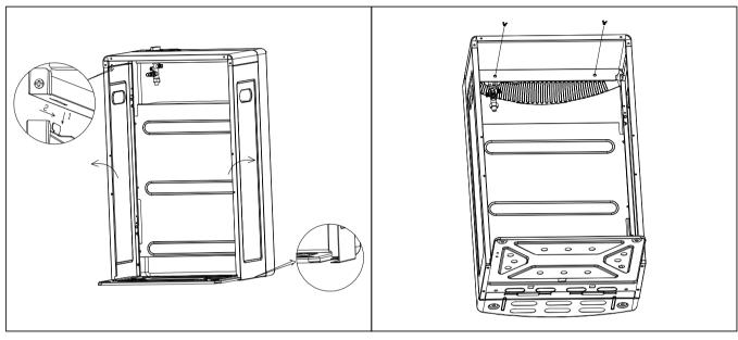
5. Match the side panel with baseplate in four holes, use the screwdriver to fix with 4pcs M5\*8 screws.
