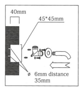
3) Dig hole for body to pipe 3.1 Hole size 45\*45mm,depth 40mm; 3.2 Dig two holes 6mm distance 35mm 3.3 Assemble spare parts as picture shows
