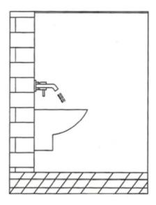
4) Connect inside pipe and test for leak checking
