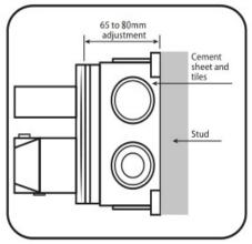
STEP 2. Attach water supply and water outlet; Screw the shower mixer assembly in place. TEST AND CHECK FOR LEAKS.
