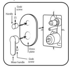
STEP 4. Install into the wall tube
