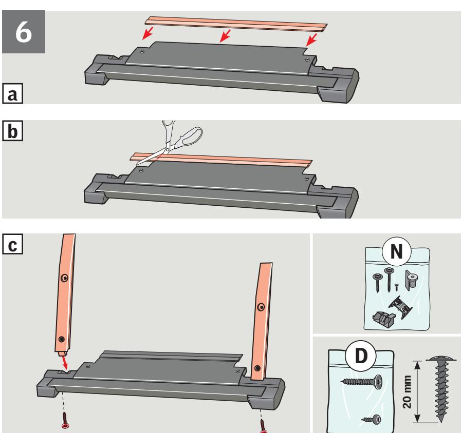
**ENGLISH:** Fit gasket on bottom cover and cut to length **a**, **b**. Fit storm brackets to connection pieces **c**.
