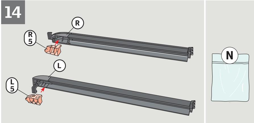
**ENGLISH:** Fit plastic insert pieces on the roller shutter side channels **a**, **b**.
