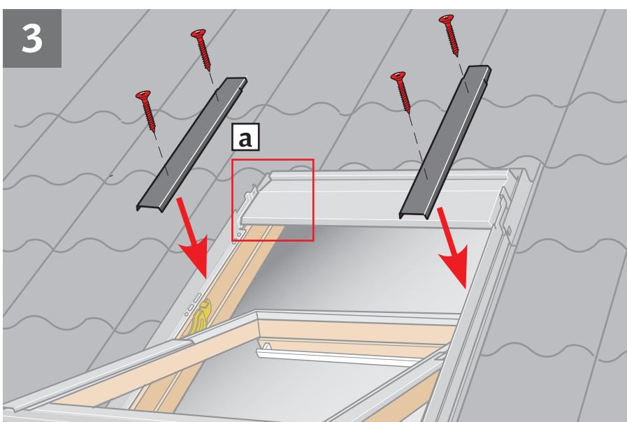
**ENGLISH:** Loosen screws in top cover **a**. Fit window covers using existing screws. Re-tighten top cover screws.
