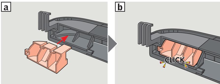
**ENGLISH:** Push side channels into position **a** and lay down on side covers **b**. Attach opening restrictors to side covers with screws **c**.
