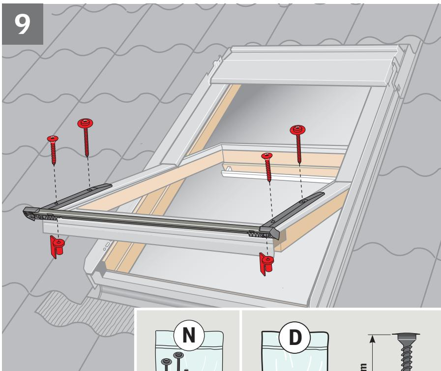
**ENGLISH:** Fit bottom cover. Secure lower screws with special nuts.
