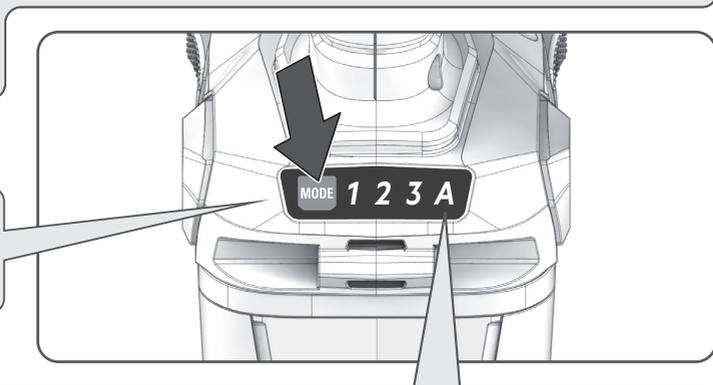
The "A" function is designed to give the user greater control in application and reduce damage to the fastener or work surface by automatically shutting the tool off after the tool senses the mechanism impacting for approximately one second.
