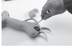
2. Remove the blade nut retaining buckle bolts (this step is essential).
