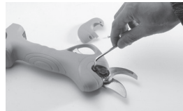
9. Insert the locking nut TAB
