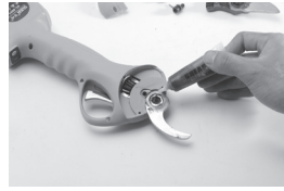
6. When replacing the blades, it is necessary to add lubricating oil between the blades.
