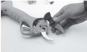
4. Disassemble the pin and remove the movable blade.
