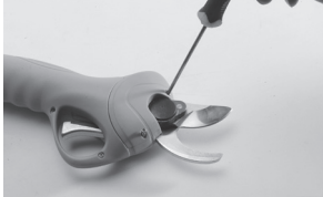
1. Remove the screws with a screwdriver and open the cover.
