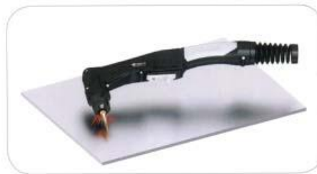
Hold the torch at an angle to the work piece, pull the trigger to start the arc and slowly rotate it to an upright position.
