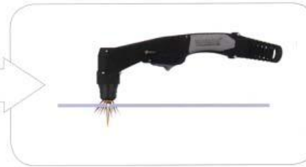
When sparks are exiting from the bottom of the work piece, the arc has pierced through the material.
