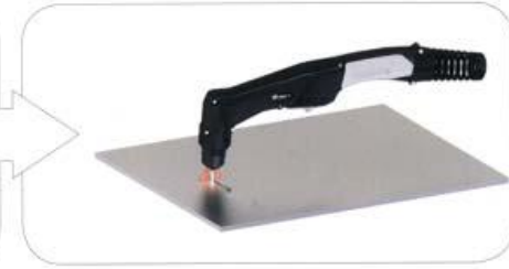
When the pierce is complete, proceed with cutting.
