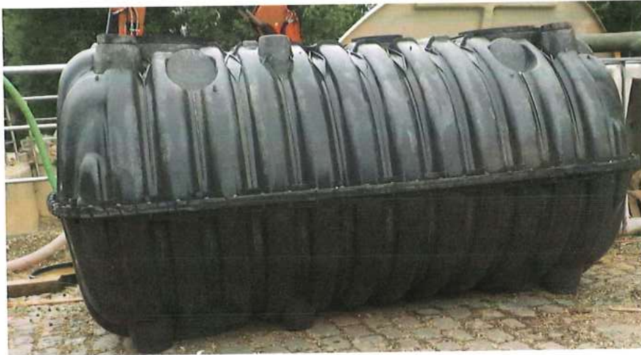
Figure 3: Tank buried out after 3 weeks of testing
