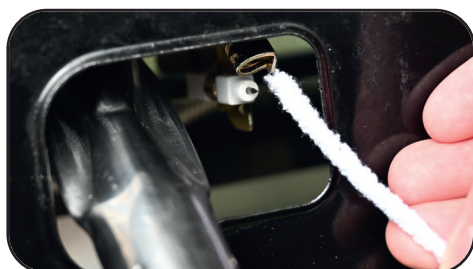
Cleaning of the pilot flame conductor with a chenille wire or a pipe cleaner.
