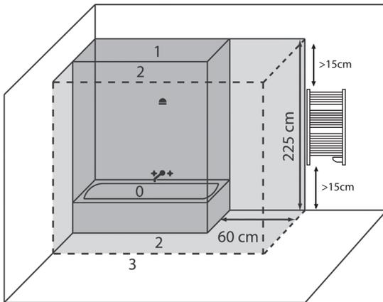
**WARNING** this product shall be installed only in the volumes 2 & 3 of a bathroom according the rules of standard installation. We suggest you to contact a professional electrician for assistance.
