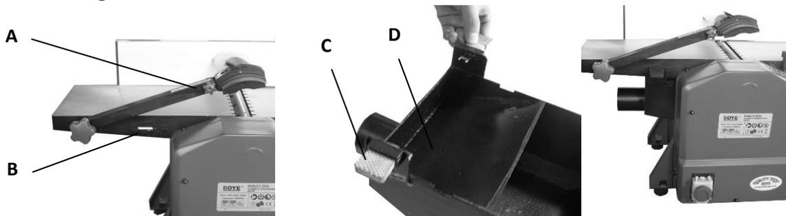
Lift up the blade arm **A** so that the longitude holes **B** being exposed; Pull out the key **C** on both sides of the dust chute **D**; Move down the thickness table to the lowest position, and insert the dust chute **D**; The dust chute **D** is so positioned that both keys **C** are in line with the longitude holes **B**. Then push both keys **C** into the longitude holes **B**.
