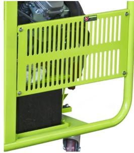
Loosen the protective cover to get access to the battery.
