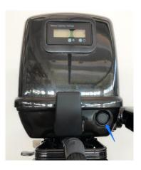
**Warning**: to avoid damages in case of collision with the seabed, turn the throttle grip to zero and unlock the motor tilt before moving the gear shift to forward.
