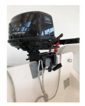
Attach a strop or retaining chain to the eyelet of the outboard if the boat has one.
