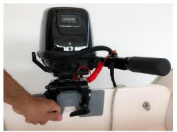
Place the outboard on the transom or outboard mount on the centreline of the boat and tighten the two clamps securely.
