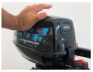
Check the fitting of the top cowling by pushing it sideways in both directions. If it is loose, have it repaired by the nearest service centre.
