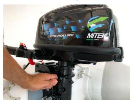
If the boat already has a rudder (e.g. sailboat), you can lock the motor in place with the side screw.
