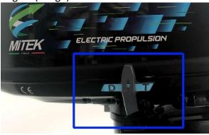
• <u>MO 15hp and MO 20hp</u>: to select the desired direction of travel, move the selector lever towards the direction in which you want to travel (image), as indicated by the FORWARD or REVERSE arrows.
