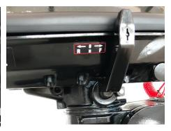
• <u>15hp and 20hp models:</u> switch off the motor, remove the safety key, set the tilt lock lever to "N" on models with tiller control, unlock the tilt by pushing down the "tilt block" lever (Figure 1), lift the engine until the tilt block is engaged by means of the appropriate lever (Figure 2). Make sure that the tilt lock is fully engaged before releasing the motor. To lower again, lift the motor slightly, operate the tilt lever and lower the motor.
