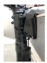
Check that the motor axis is perpendicular to the water and if necessary move the pin to achieve the correct inclination (trim).
