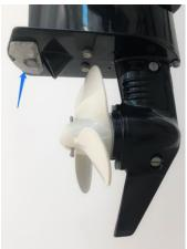
Inspect the external anodes periodically and remove scales from the surfaces of the anodes.
