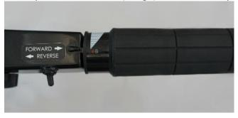
**Warning**: keep the gear shift lever in DRIVE for forward or reverse and set it to TILT to raise the engine (image).
