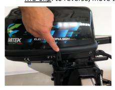
F = Forward N = Neutral R = Reverse • MO 9.9hp: to select the desired direction of travel, move the selector lever towards the direction in which you want to travel (image), as indicated by the FORWARD or REVERSE arrows.
