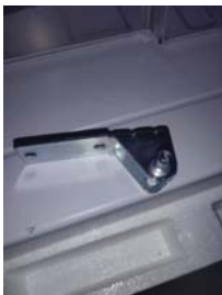
Step 5: remove the lower hinge
