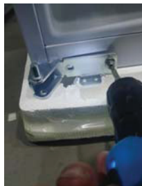
Step 7: fix the lower hinge on the opposite side
