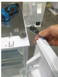
Step 2: put the foamed door aside and remove the door
