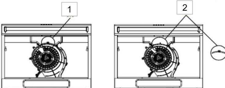
Do not remove the mode selection block (**Fig. 1**) for exhaust air operation.
