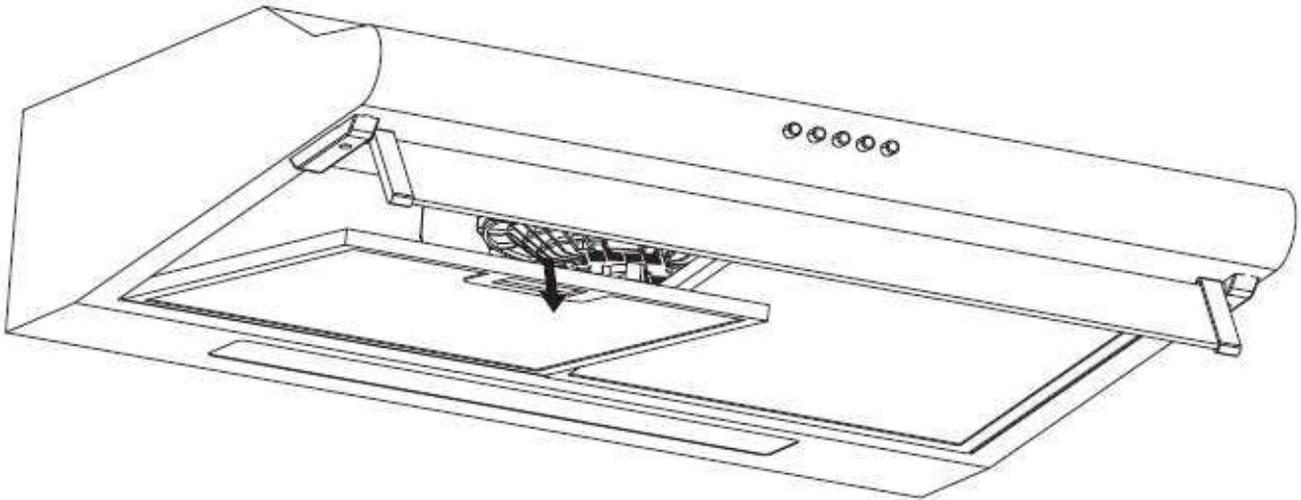
3. Rotate the LED bulb in direction shown in below Fig. Replace it by new one.
