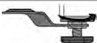
3. Turn the adjustable feet for horizontal alignment.
