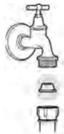
5. Reinstall the water inlet filter in the hose end. Ensure that the seal (rubber washer) is properly inserted in the valve connection.
