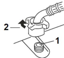
**NOTICE!** Do not overtighten the water inlet hose. Overtightening of the water inlet hose can damage the water inlet valve.
