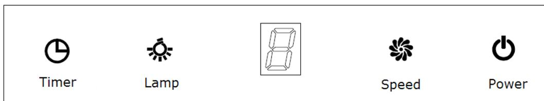
1. Press the “Power” button, the button control the “on” & “off ” of the hood.
