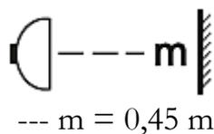
Required minimum distance to surfaces such as pot lids, oven cloths etc. to avoid any hot parts and risk of fire.
