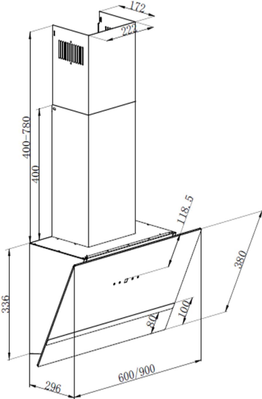
Abmessungen in mm.
