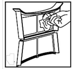
6. Insert the fluff filter properly (**the fluff filter must be dry completely**).
