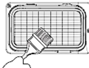
4. Reinstall the condenser properly and close the locks. **The condenser must be completely dry before reinstallation.**
