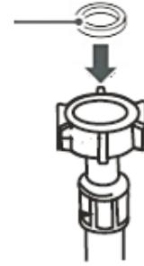
2. Attach the **straight** end of the water inlet hose to the appropriate water connection (s. fig. on the right).
