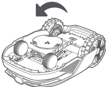
4. Clean the housing, blade disc and chassis with a hose.
