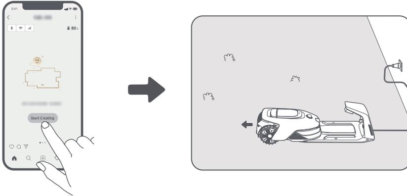
② Guide the robot to the edge of your lawn and tap **Set Starting Point** to establish the starting point for the boundary.
