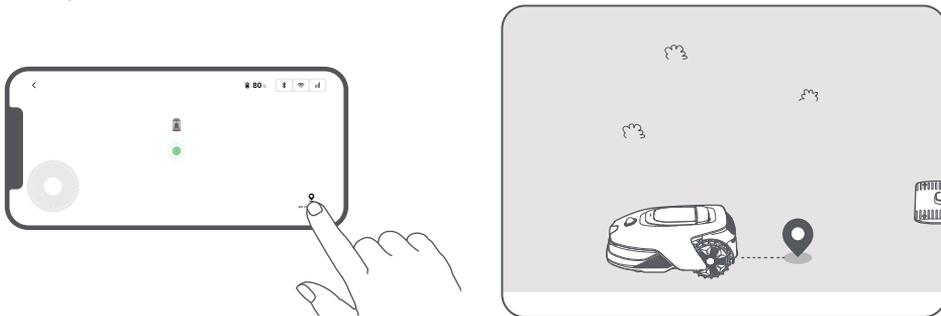
③ Remote control the robot to move along the perimeter of your lawn to map out the work area. During the mapping process, please bear in mind:
