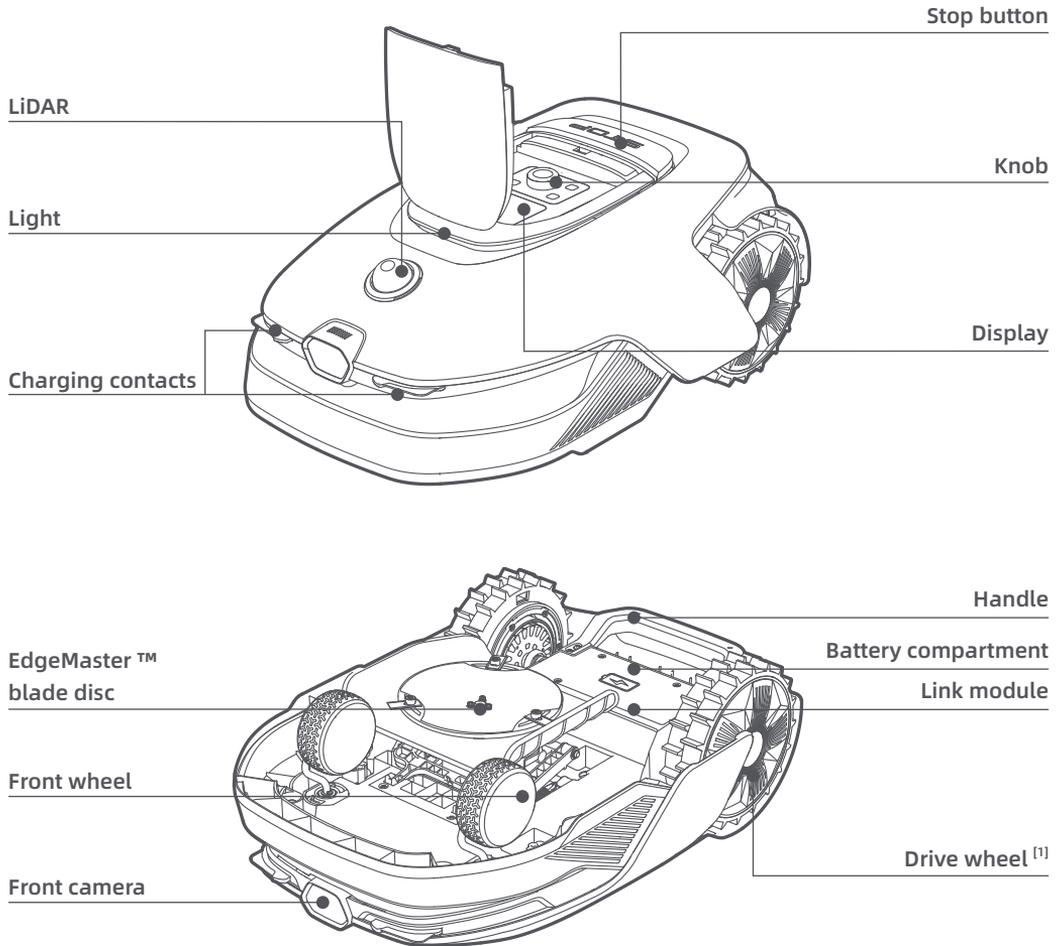
[1] Equipped with hub motors.
