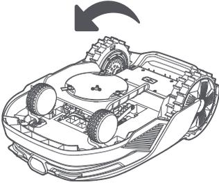
5. Remove the blade by aligning the hole of the blade with the shaft.
