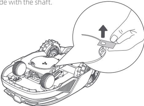
7. Press the button under the blade disc and align the hole of the holder with the shaft to fasten the holders and the blades.
