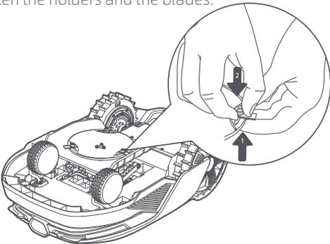
4. Remove the holder by pressing the button under the blade disc.
