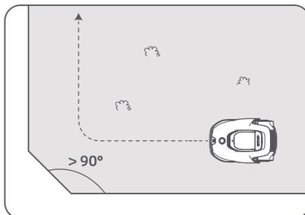
4 When the robot returns to within **1 m** of the starting point, you can tap **Close Boundary** and the boundary will automatically be completed.
