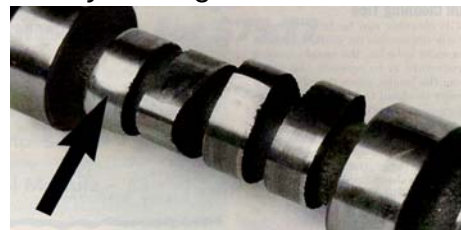
Image 1: Worn Cam Lobe with Engine Oil Only
