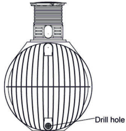
Fig. 31: Interconnecting multiple tanks – PROFI
