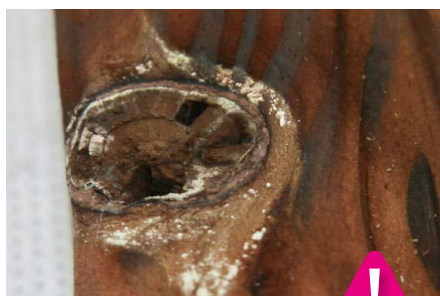
Knot breakouts – up to 20% permitted in intermittent cases
