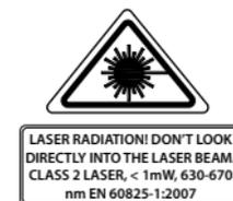
**Class laser, with a 630-670 nm wavelength and in accordance with DIN EN 60825-1: 2007. Do not look directly into the light beam of the measurement device and do not use other optical instruments when using this device. The above mentioned information agrees with the warning label from the device.**
