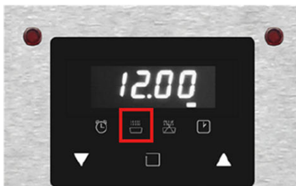
Cooking duration symbol: select this symbol when the oven should heat for a set time.
