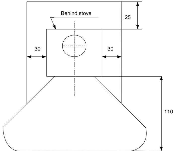
It is possible to reduce the distance to flammable material by insulating with at least 5.0 cm insulation with identical properties to Aduro Superisol, Isolrath 1000 or similar material around the Aduro 5-1. Please make very sure that there is still at least a 2.5 cm space around the Aduro 5-1. This means that the distance to flammable material can be reduced to 7.5 cm (2.5 cm space around the insert + 5 cm insulation).
