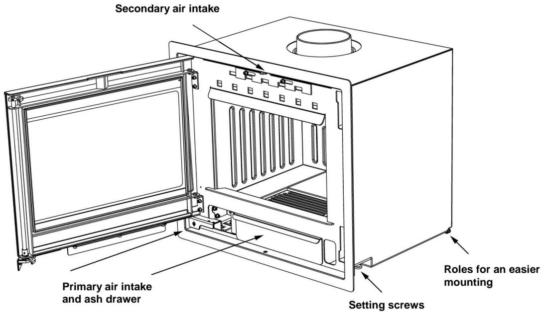
\* Remember to mount the set screws before the insert is placed at the correct position. The set screws are in the ash drawer.
