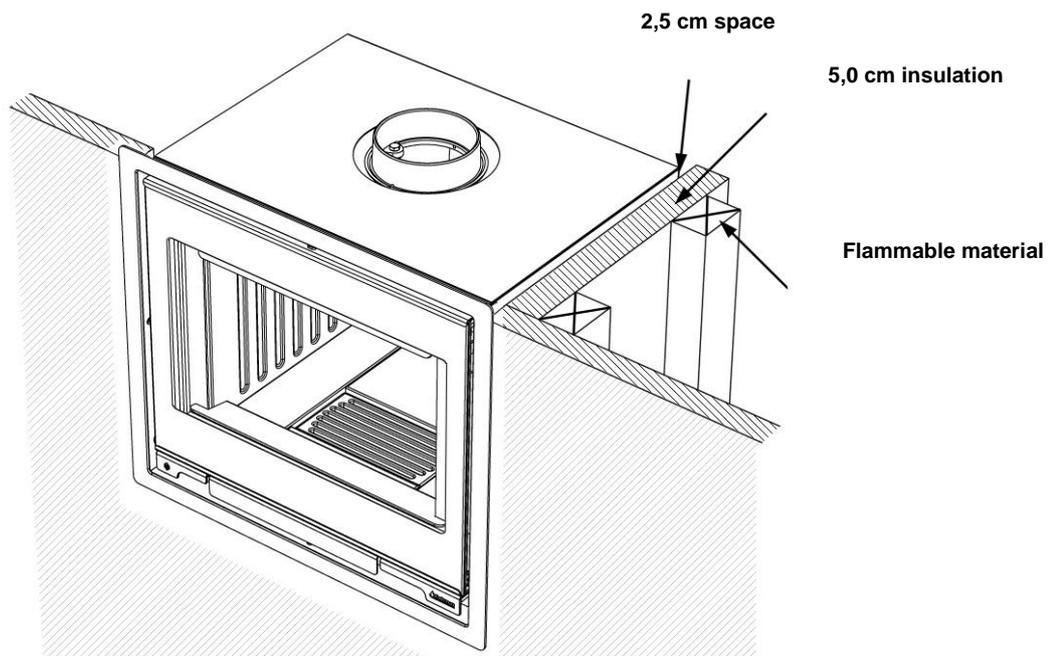
Please note: that the Aduro 5-1 must be installed on a floor with the adequate load-bearing capacity. If the existing construction does not meet this requirement, appropriate adaptation measures must be taken (e.g. a load-distributing plate).
