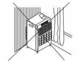
5. DO NOT position heater close to walls, furniture, net curtains, bed linen or any flammable materials as this could result in a risk of fire. The following minimum distances should be respected: 50 cm from the sides and 100cm from the front. ALWAYS face the heater towards the centre of the room. The heater should be positioned on a level surface at all times.
