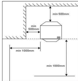
Note: Minimum distance from mobile heater to the ceiling at least 1000mm.
