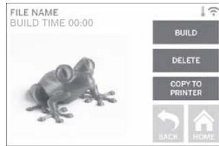
5. Your 3D40 FLEX will first align the extruder and build platform to their zero positions then the level sensor will lightly touch the build platform to complete alignment. Your extruder tip will begin to heat which may take a few minutes. Once the proper temperature is reached your model will begin to build.
