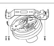
**1.** Locate and mark the centre of the joist, pass the supply wires through the hole in the supporting bar, secure to the ceiling joist by using the spring washers, flat washers, and the 50mm wood screws.
