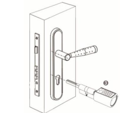
4. Fixate cylinder in the lock with a centering screw.
