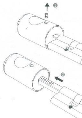
3. Insert cylinder into the lock. The position of the cylinder in the lock is correct when the latch can be operated via the spindle of the cylinder.
