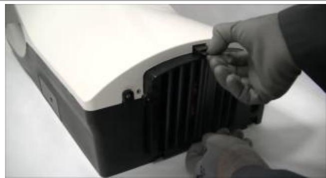
*Remove the filter assembly by unclipping it from the base.*
