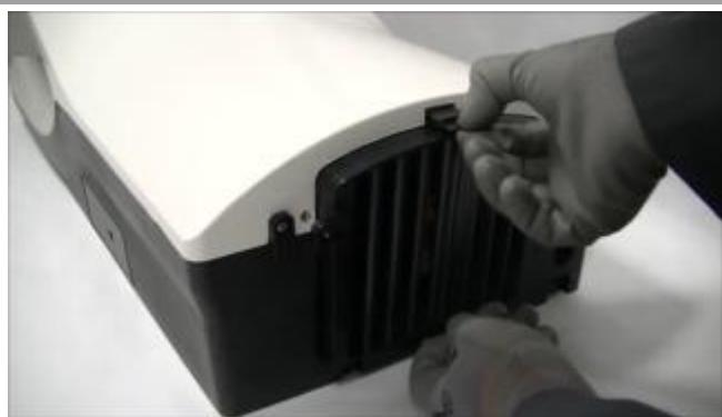
*Remove the filter assembly by unclipping it from the base.*
