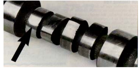
Image 1: Worn Cam Lobe with Engine Oil Only
